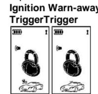
Clear the Flash Icon and Melody Sound: Cycle ignition then press the button first, within 3 seconds press and \* buttons at the same time. It will clear the flash icon and melody sound on the LCD screen transceiver
